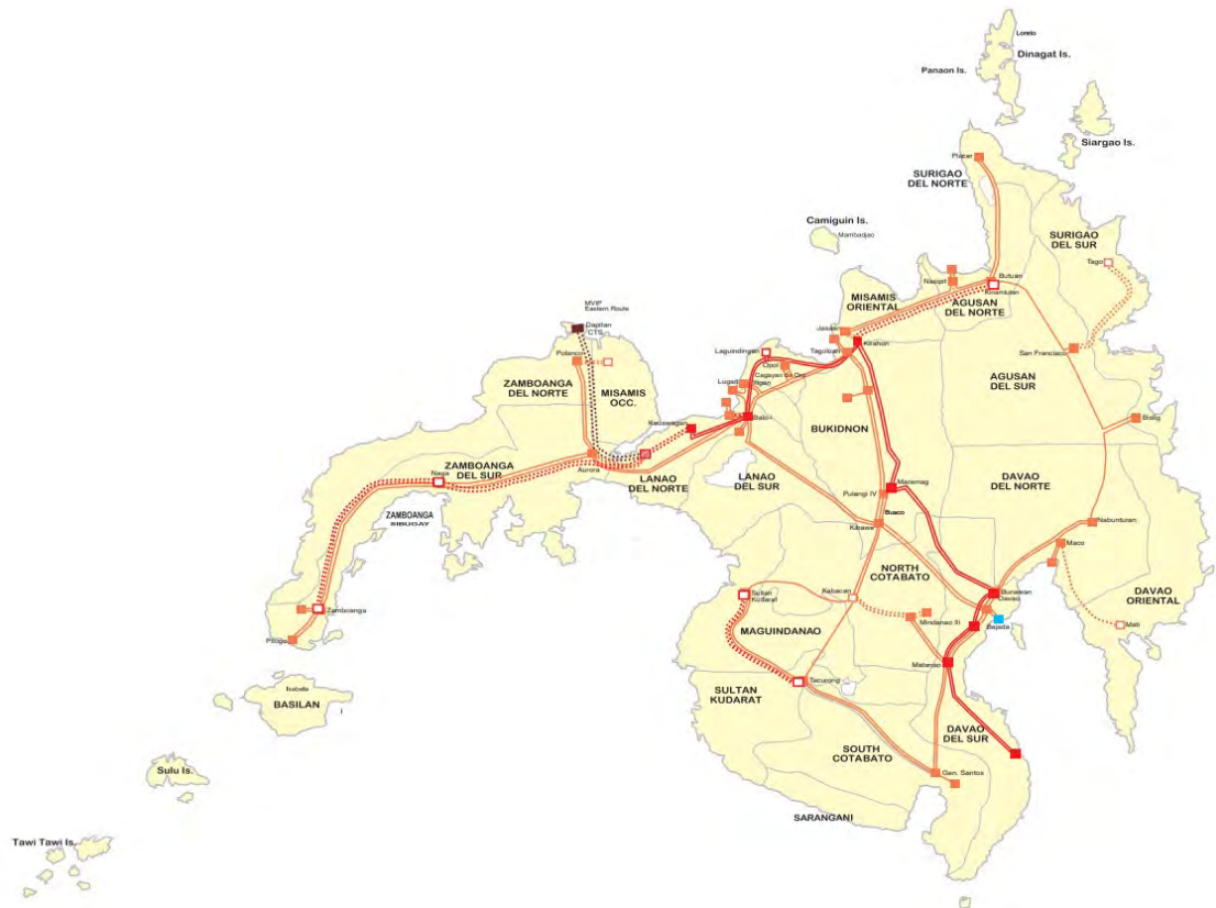
Figure 23: Mindanao Power Grid
